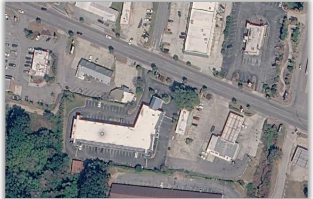
Due to a lack of coordination, each building has its own standalone parking lot, some of which do not connect to each other, all laid out in an illogical manner.
